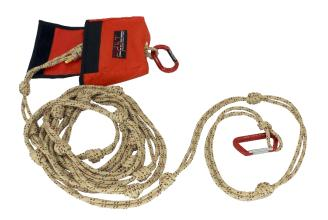
The haul line is 75' of 7.5mm bail-out compliant, heat-resistant rope, double-overed, and knotted every 12" to 16" for positive handholds and mechanical advantage. The total length of the tied rope is approximately 22'.
