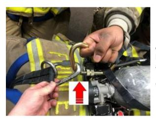
Deploy the upper lashing strap with the oversized "D" carabiner and the lower lashing strap with the tri-link (An "O" ring is attached to the tri-link as a grab ring.)
