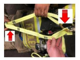
Secure the handle with the oversized "D" carabiner on the upper lashing strap. Pull on the opposite side of the Multi-Loop Strap to tighten the straps and then secure the Multi-Loop Strap using the loops to the oversized "D" carabiner. Tighten the system.
